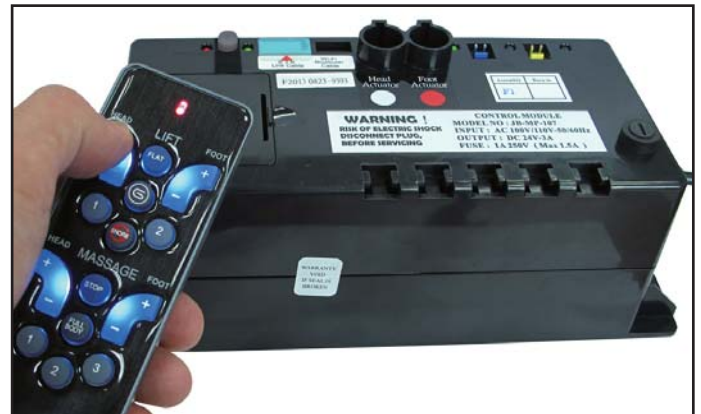
Figure 2: A flashing Green LED indicates the control box has received the remote control signal.
