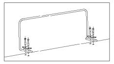
**NOTE:** Use only a manual screwdriver to install the retainer bolts. DO NOT use a power screwdriver to tighten the bolts.
